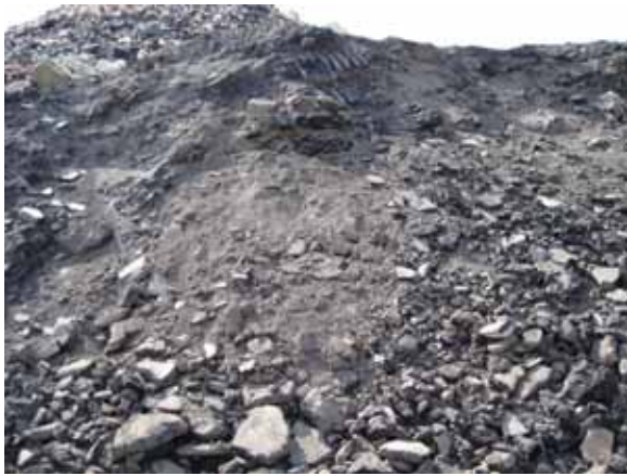
Figure 4 – Reclaimed asphalt for crushing
