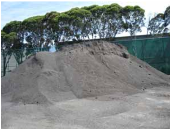
Figure 5 – RAP after processing
