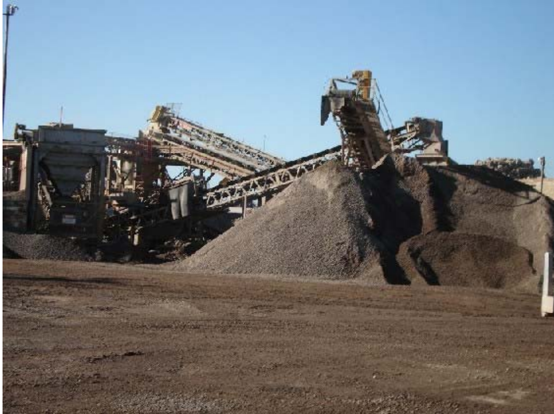
Figure 4: Crushed rock (20 mm) stockpile - Alex Fraser Recycling, Laverton
