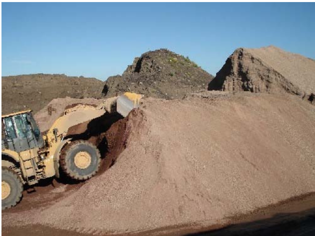
Figure 1: Crushed brick (20 mm) stock pile - Alex Fraser Recycling, Laverton
