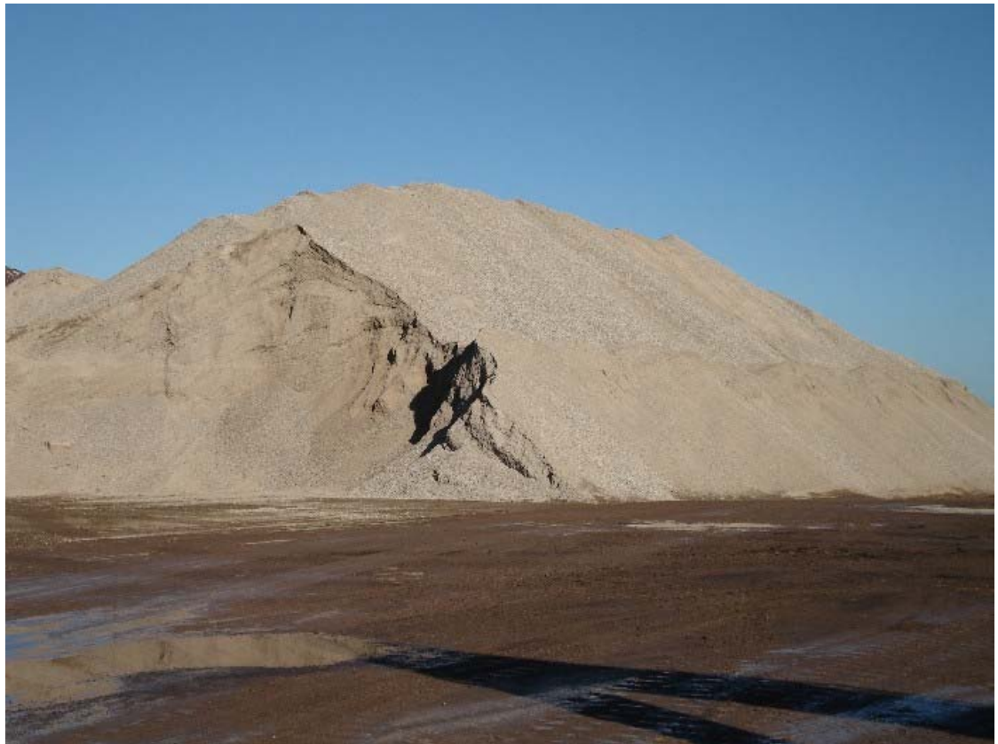
Figure 3: Crushed concrete (20 mm) stockpile - Alex Fraser Recycling, Laverton
