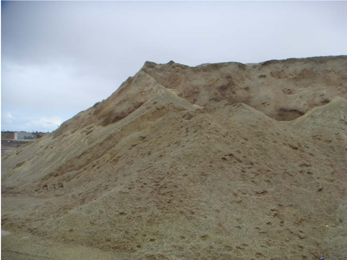
Figure 2: Crushed glass (5 mm and smaller) stock pile - Alex Fraser Recycling, Laverton
